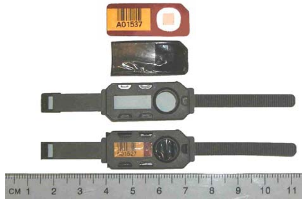
Figure 5. EXTRAD-100 Finger ring thermoluminescent dosimeters at various stages of assembly.
