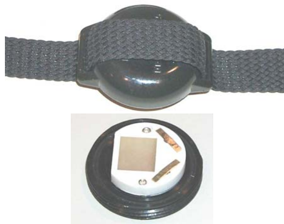
Figure 9. Marine Corps DT-236 battlefield dosimeter; (Top: On wristband, Bottom: Opened up).
